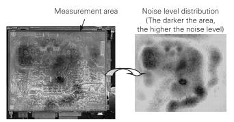
Fig. 4: PCB of a prototype production machine (before countermeasures)
