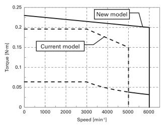
Fig. 3: Torque vs. speed characteristics (SANYO DENKI amplifier combination, 48 VDC)
